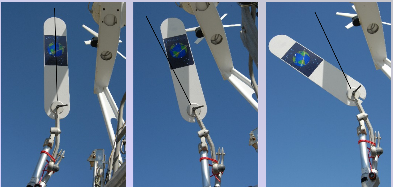
Wind vane settings depending on wind strength. Left: Standard setting for most winds. The wind vane follows the line of the pendulum arm shaft. Center: Light wind setting, not provided by the manufacturer at the time but proved to be helpful and effective. The wind vane is virtually pre-balanced in light winds. Strong wind setting. Depending on the wind the vane should be tilted out of the wind. Some sailors have simply sawed a smaller wind vane out of spare plywood as an alternative. Wilfried Erdmann, for example, did this on his Aries. The black line illustrates the extension of the pendulum arm shaft axis in each case.
