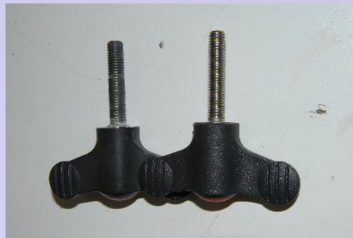
Clamping screws or handles, old and new. Noticeable: the protruding steel pin of the old screw (left).
