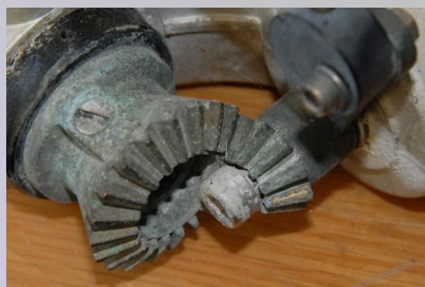
Here is the heavily soiled bevel gear just before dismantling. We had lost the cover and didn't pay much attention to the system in the first year after sailing around the world. After thorough cleaning, the bronze parts showed virtually no wear!
