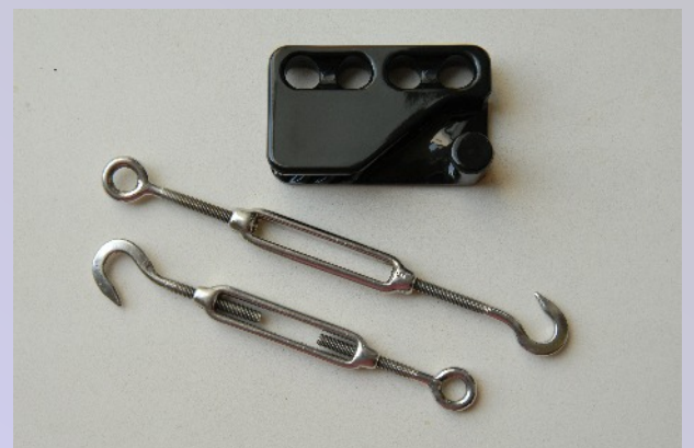
Below are the tensioning screws we used to adjust the line tension. The manufacturer later recommended a fender clamp (above) as the best way to reduce line play. He said that one is enough, regardless of which of the two pull lines it is used on. We suggest our solution as the easiest way.
