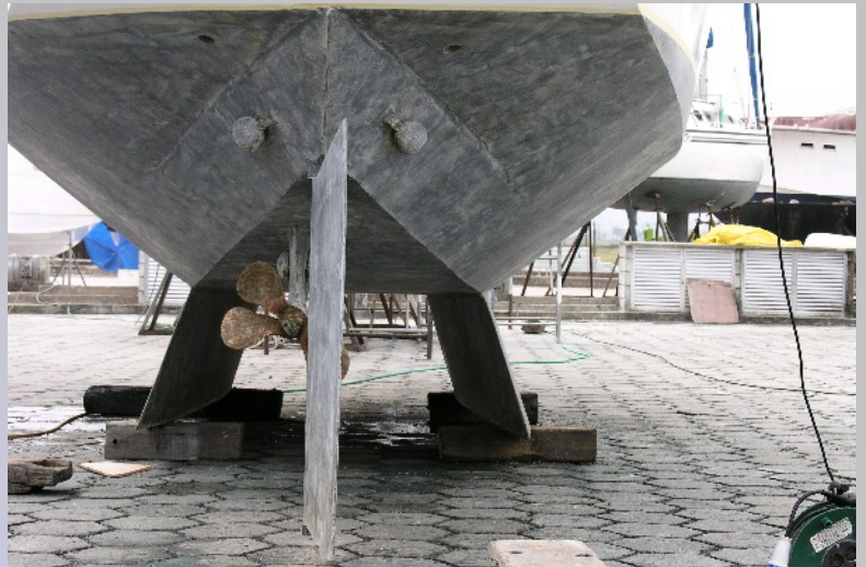
JUST DO IT after the underwater hull has been freshly brushed with a stainless steel pot brush and angle grinder. Whether for activation or as preparation for a new layer of paint, the result always looks the same. Also to see: the shaft with the Autoprop can be pulled past the rudder without any problems thanks to the offset arrangement of the shaft sleeve and the skeg.
