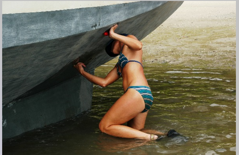
After cleaning the hull, Anke inspects the through-hull fittings. These also need to be cleaned, of course.
