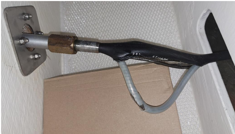
Pic 1: Cause of all the work was an Orca attack on 01/05/23 near Barbate, Spain. This pic shows the damage of the aft steering cable.
