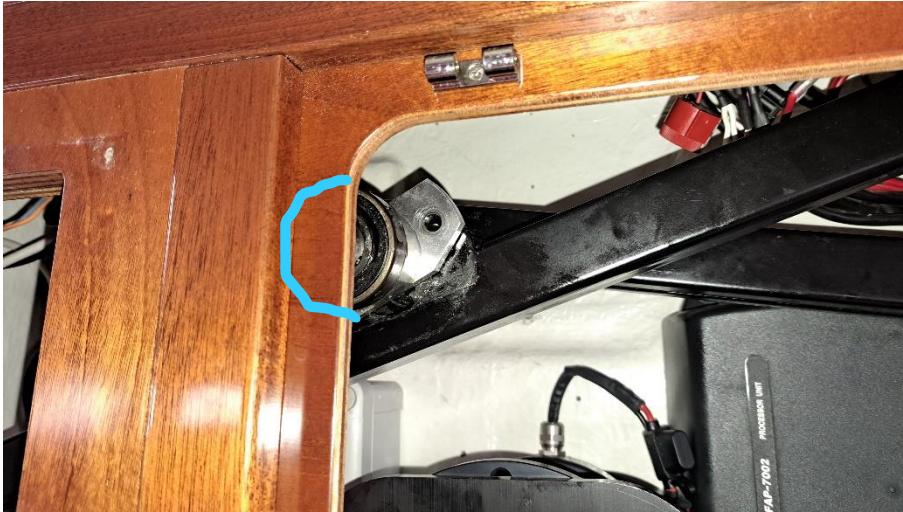
Pic 4: This nice problem causes a lot of additional work: No chance to pull the axle to the front side, except you cut the wood work or you use a saw.
