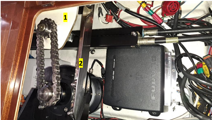
Pic 5: Jeffa autopilot (rotary drive), the chain, front support of the axle (#1) and support strut (#2)
