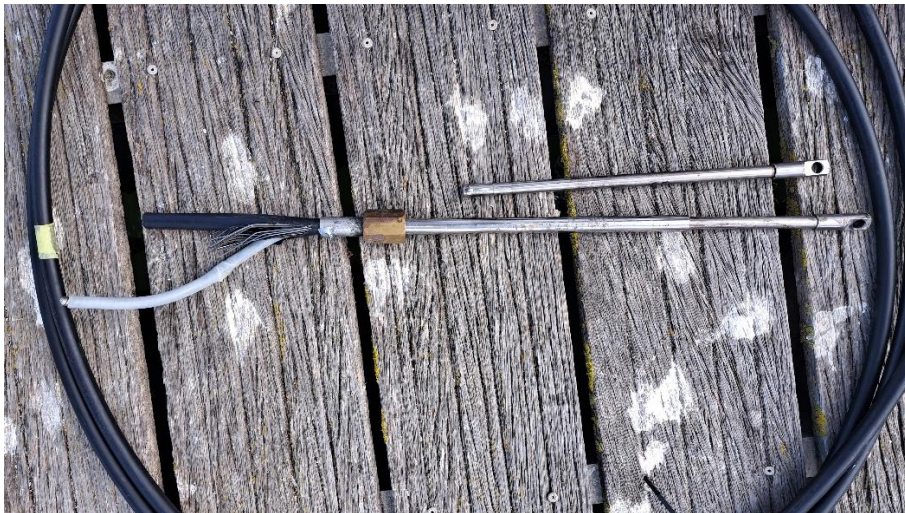
Pic 2: First we cut the aft steering cable. Later we figured out, that the second cable was damaged too. The push rod was pulled off the inner cable.
