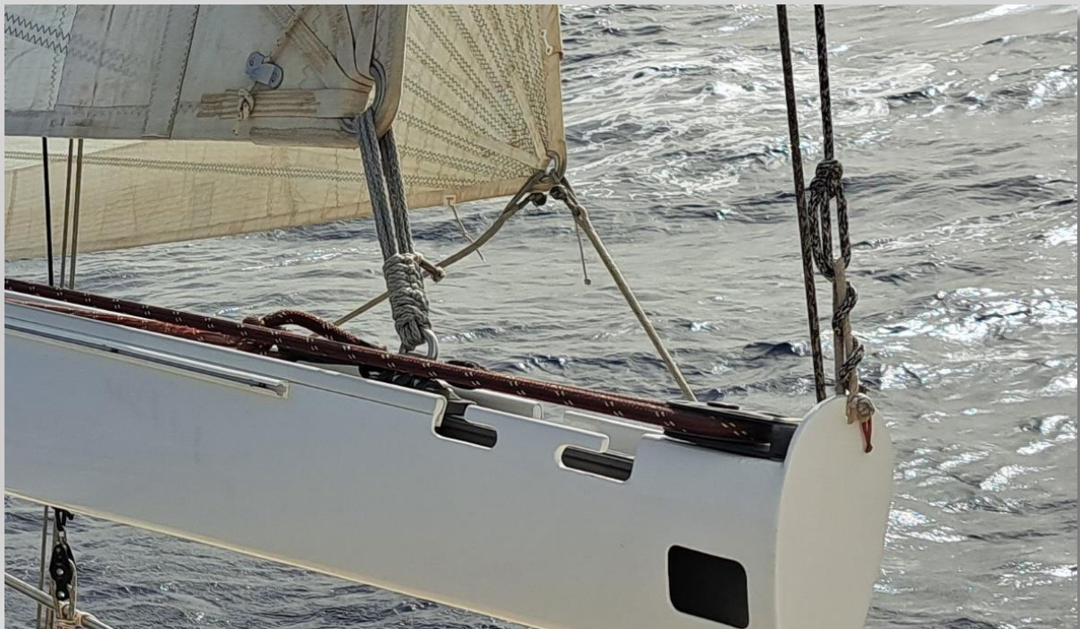
The mainsail clew on MAGO DEL SUR. Only lashed. The ball-bearing traveller of the outhaul is not visible, only the eye for the lashing. The outhaul line is guided over the reel on the boom nock.
