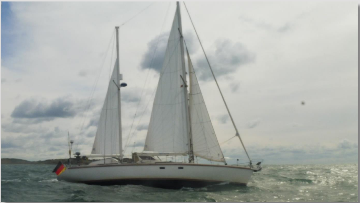
MAGO DEL SUR in August 2018, slightly blurred in rough seas on the Baltic Sea. Not easy to recognise: The main is reefed by one batten and the mizzen by two. (Foto: Manfred, SY FATU IVA)
