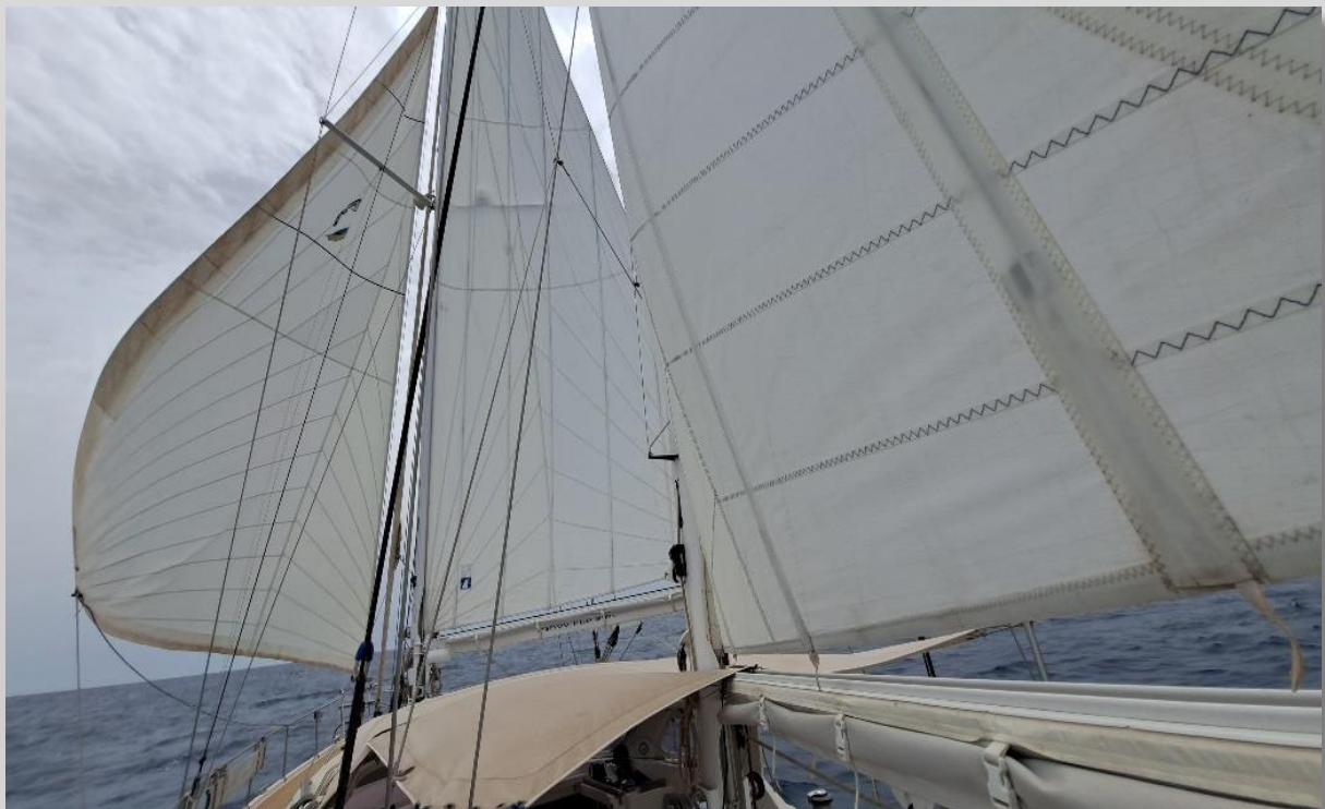
This also works: double butterfly. Here genoa to port, main to starboard, mizzen sheeted like the genoa on the port side.
