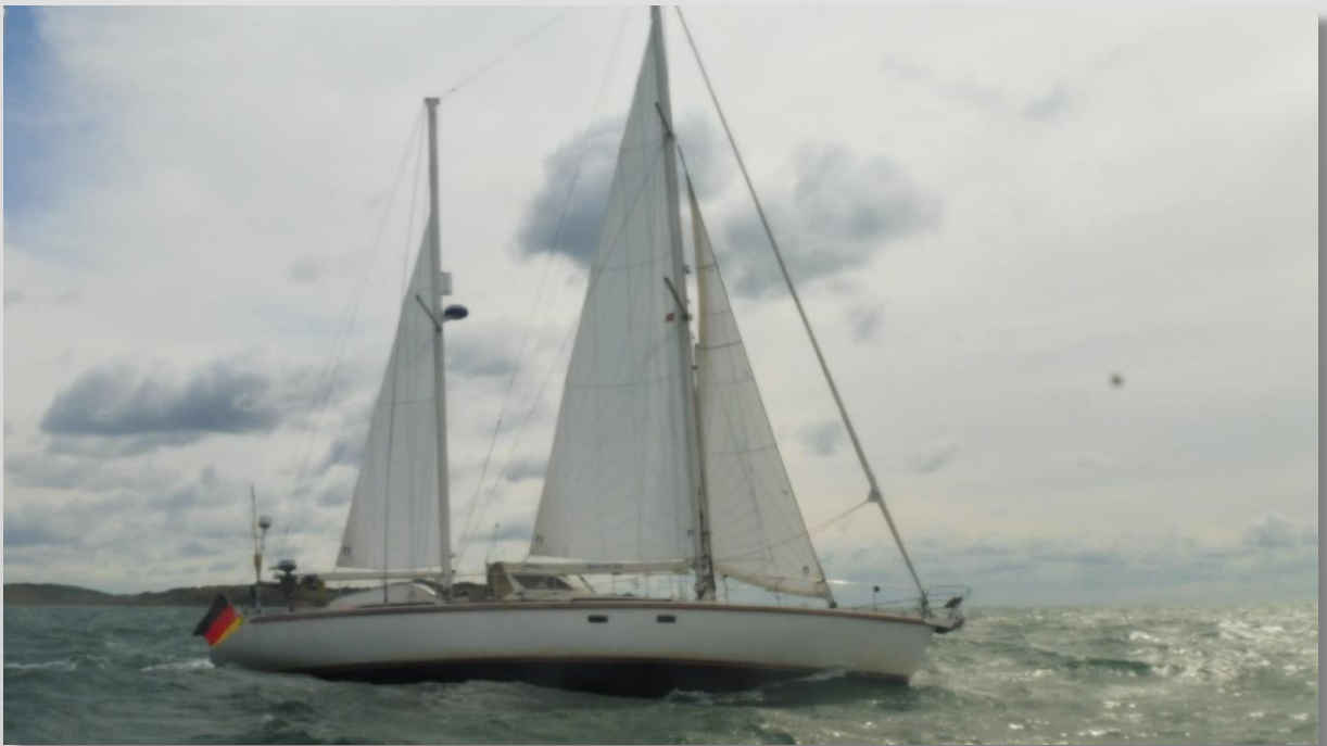
MAGO DEL SUR in August 2018, slightly blurred in rough seas on the Baltic Sea. Not easy to recognise: The main is reefed by one batten and the mizzen by two. (Foto: Manfred, SY FATU IVA)
